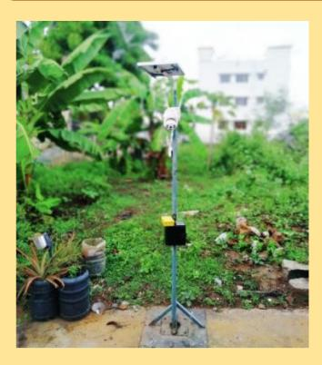
V. Shanmugam, T.S. Surendiran, M.L. Sanjay, M. Tharunkumar of EEE – IInd Year developed a Wireless solar power CCTV suitable for both remote and urban location.24/7 can be monitored by app.
