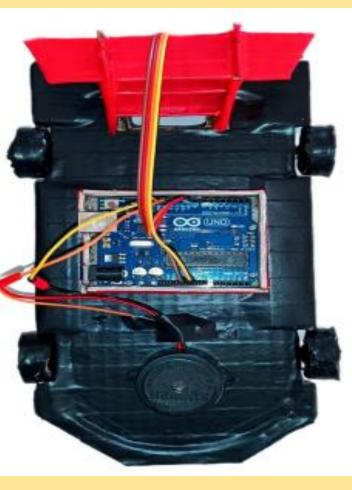
When we take reverse in car we may crash into something. To avoid this we created this Project. So by using this alert if any Obstacle is behind to our Car within a distance of less than 20 cm the ultrasonic sensor deduct the distance and the buzzer alert us. By hearing the alert we may know something that could be in the distance of <20cm and We need to drive and park the car according to the distance.
